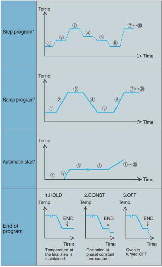
\* The number of repetitions of a program can be preset between 1 and 999. Stepwise damper setting is possible.
